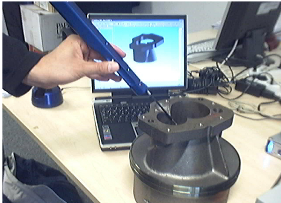
Digitization of a pipe flange
