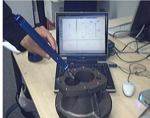
Inspection at a pump
