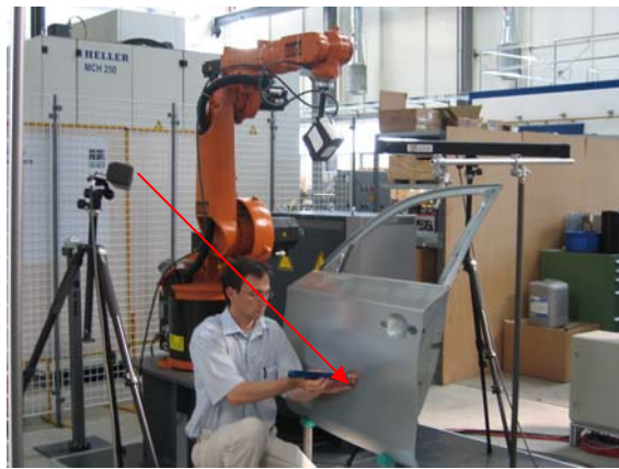
3D Creator DUAL – taking measure points
